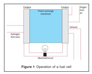
where a chemical reaction strips them of their electrons. The hydrogen atoms are now 'ionized', and carry a positive electrical charge. The negatively charged electrons provide the current through wires to do work. If AC (alternating current) is needed, the DC output of the fuel cell must be routed through a conversion device called an inverter.
